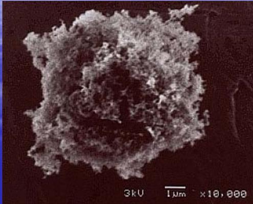
**An electron Microscope Image of a Black Carbon Soot particle (4).**
