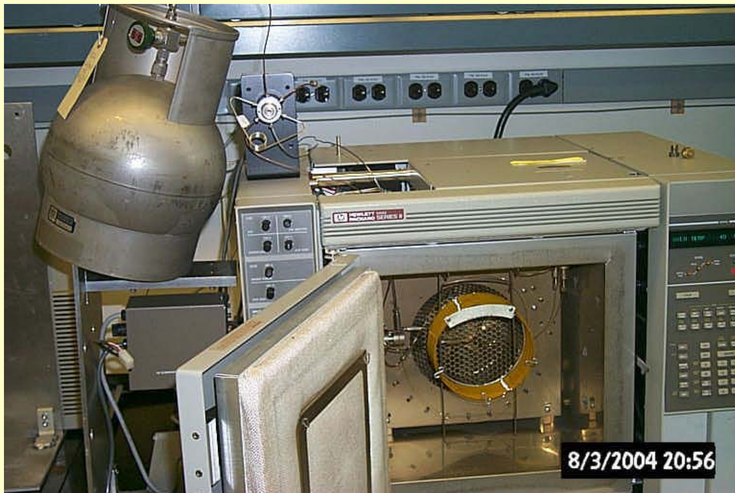
GC with Flame Ionization Detector ( \text{CH}_4 ) and Electron Capture Detector ( \text{N}_2\text{O} )
