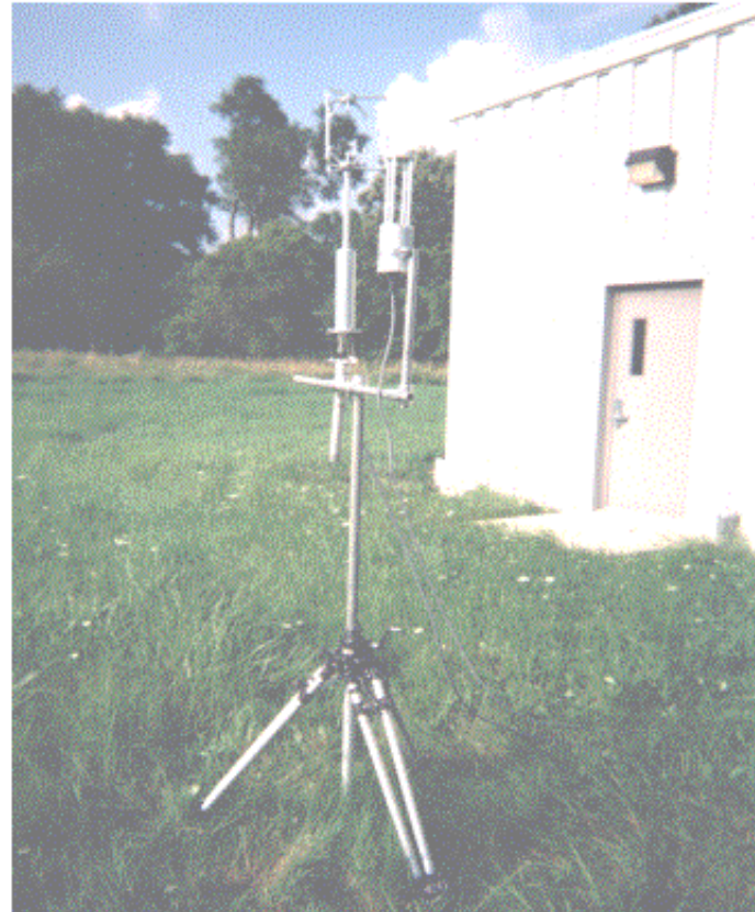
A portable eddy covariance system has recently been built and tested for future experimental use.
